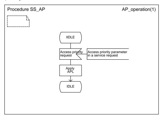
Figure 1: SS-AP supplementary service, overall MS SDL
